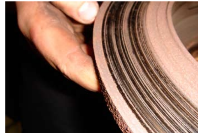
A worn ZJ rear brake disc found on a brake inspection.
