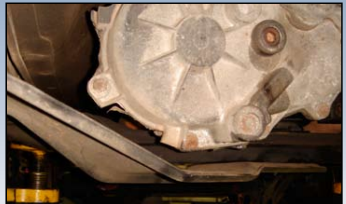
Transfer case is now clearing the bash plate with the new mount fitted
