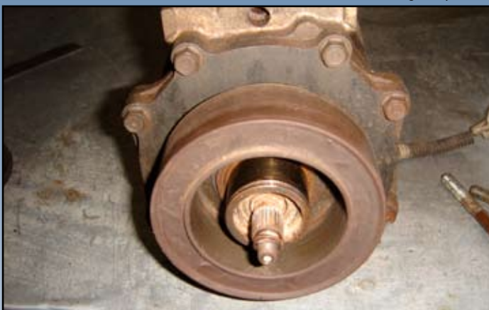
Clutch face assembly removed from the compressor
