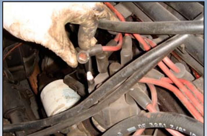
Corroded distributor cap post
