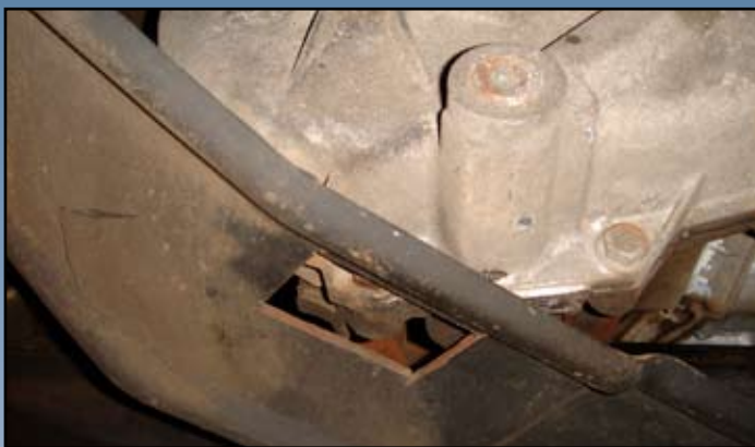
Hole cut in transfer case bash plate
