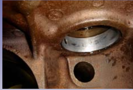
A badly worn camshaft bearing
