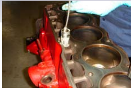
New lifters being fitted
