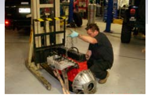
Manifolds, bellhousing and clutch fitted to motor and Travis prepares the motor to be lifted into the engine bay
