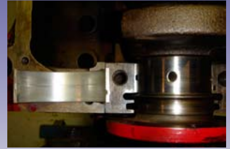
The rear main bearing cap was good to reuse
