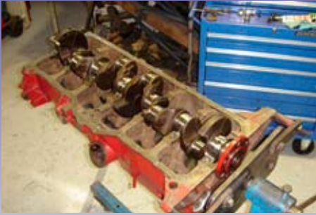
Motor stripped ready for the crankshaft to be removed
