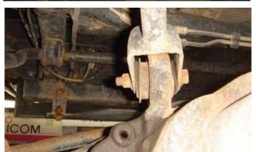
The bent rear panhard and no front panhard was contorting it's control arm bushes badly at full droop. It's so important to do every aspect of a lift kit to get it right and make it last. If you lift it you need to bump stop it, extend sway bar links, brake lines, drop or lengthen panhard rods and set up caster angles. These bushes will be dead soon and this Jeep has only 24K on the clock.
