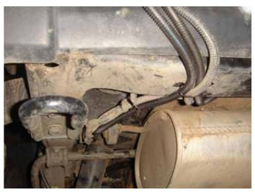
The "auto electrician" had run all the trailer loom under the cross member, the thing you slam on the ground, bump off and jack up from. We had to refit the lot to hide it and protect it from damage, this is simple stuff that should be done right first time.
